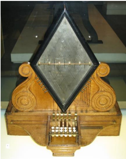
Left: William Fothergill Cooke and Charles Wheatstone's electric telegraph "needle telegraph") from 1837 now in the Science Museum. Image licensed by GNU license Via Wikimedia Commons.
