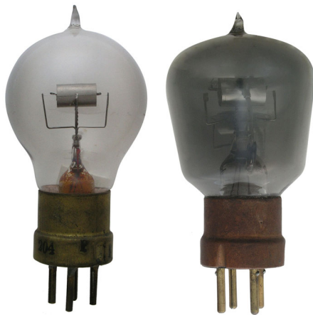
Fig. 10a & 10b: French TM and Osram F valve. The TM was a general-purpose valve used mainly as a detector or an AF amplifier. The F was a low-power transmitting valve similar in construction to the TM.
