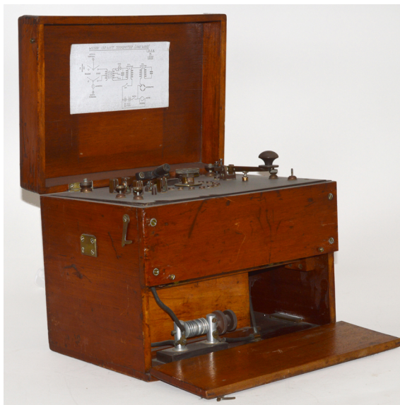
Fig 8: W/T trench Set 130-watt Wilson. Transmitter only; used with Tuner Short Wave Mk. III.
