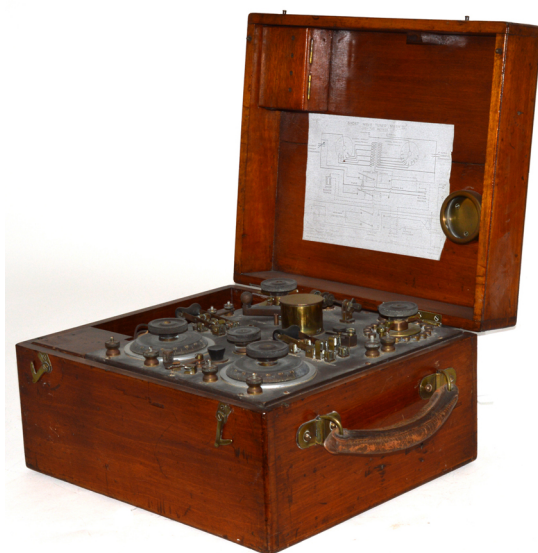
Fig 9: Tuner Short Wave Mk. III*. This receiver has both a carborundum and a Perikon detector.
