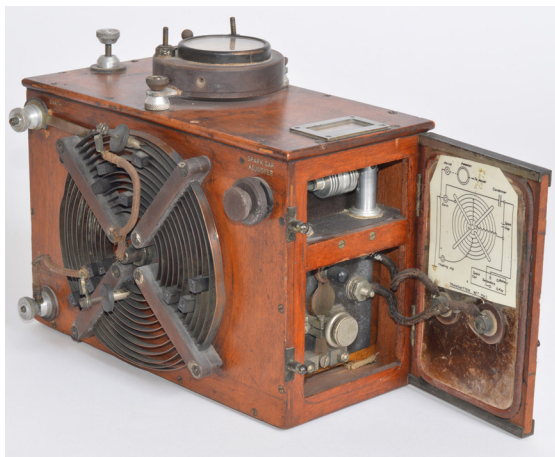
Fig 6: No. 1 Aircraft Transmitter Spark. 30-watt input. Note the spark gap on the top right inside the cabinet with the adjustment for the gap at the front.
