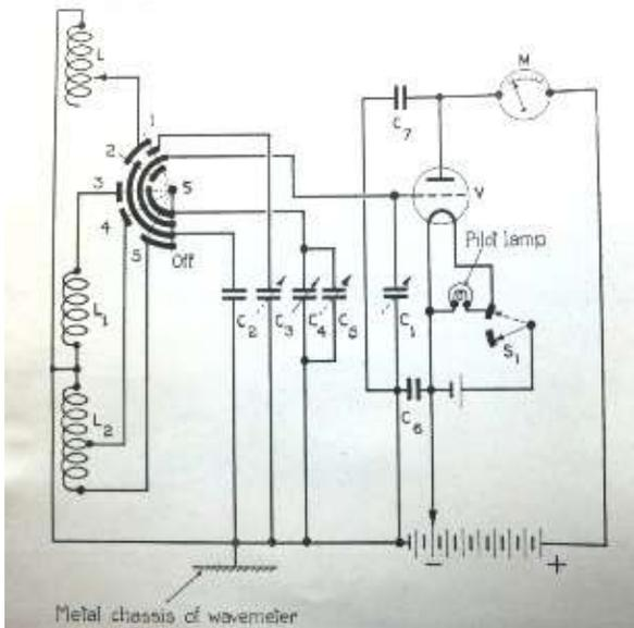
Figure 16. W1081 circuit diagram (135-500kHz & 3-15MHz)
