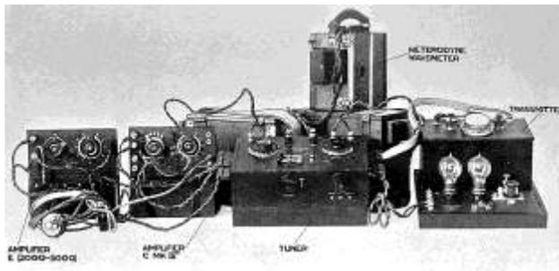
Figure 4. Army W/T set field 60W set with wavemeter [9]
