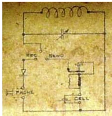
Figure 5. (a) Forward Sets B wavemeter, 65m and 80m (b) circuit diagram as shown inside lid
