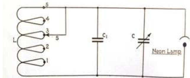
Figure 13. Circuit of W66
