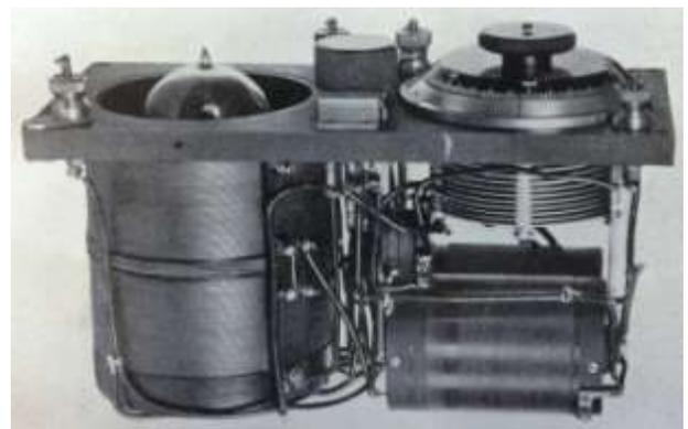
Figure 9. Circuit and internal view of Syntoniser, 300-2500 metres
